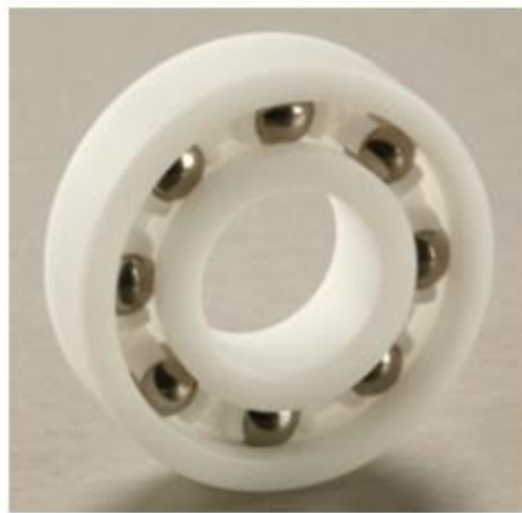
Figure 2. Polyacetal (POM) ball bearing used for Acoustic Emission Analysis.
